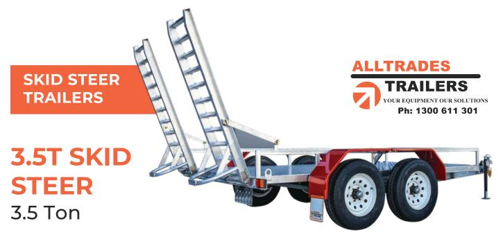
The All-Tow Skid Steer Trailer is built to suit machines with an operating weight of 2660kg or less including bucket.
